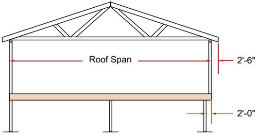
The tables and details on pages 10 and 11 indicate the type of reinforcements, if any, that are required for load-bearing cantilevers up to a maximum length of 2'-0". Cantilevers longer than 2'-0" cannot be reinforced. **However, longer cantilevers with lower loads may be allowable without reinforcement. Analyze specific applications with the BC CALC® software.**
