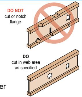
BCI® Joists are manufactured with 1 1/2" round perforated knockouts in the web at approximately 12" on center. Minimum distance from support, listed in table below, is required for all holes greater than 1 1/2"
