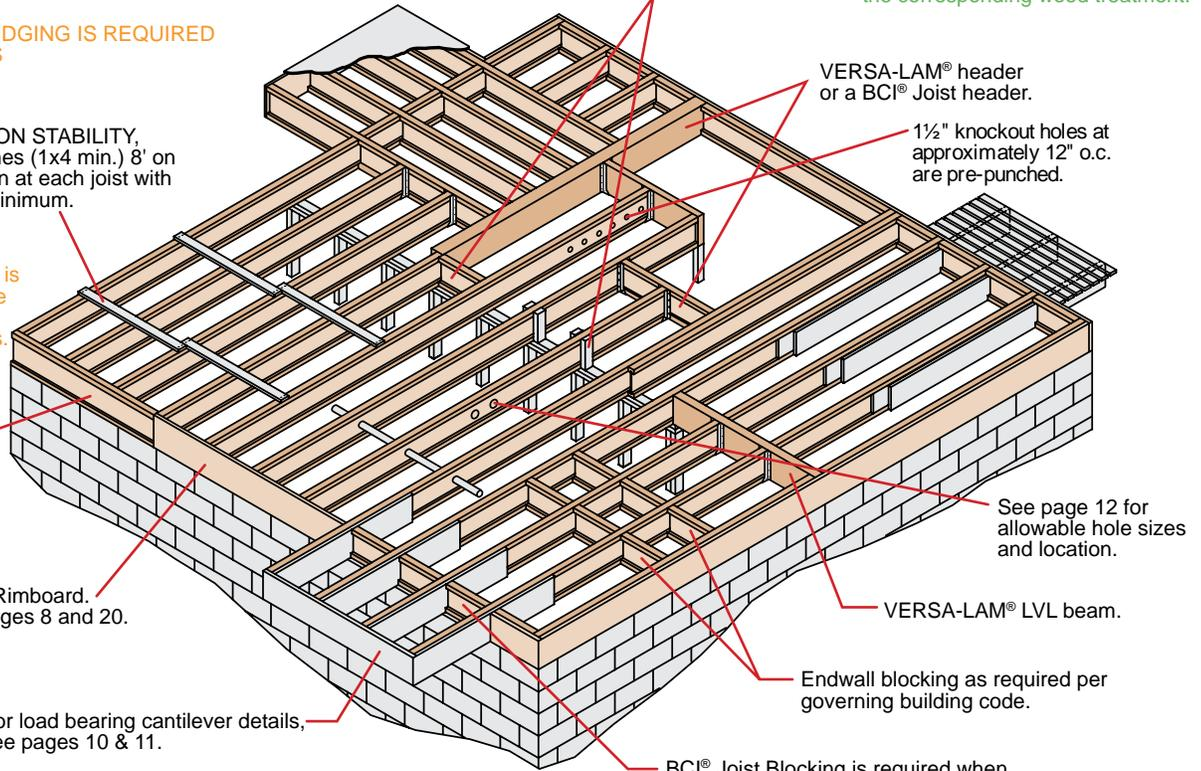
BCI® Joists, VERSA-LAM® and ALLJOIST® must be stored, installed and used in accordance with the Boise Cascade EWP Installation Guide, building codes, and to the extent not inconsistent with the Boise Cascade EWP Installation Guide, usual and customary building practices and standards. VERSA-LAM®, ALLJOIST®, and BCI® Joists must be wrapped, covered, and stored off of the ground on stickers at all times prior to installation. VERSA-LAM®, ALLJOIST® and BCI® Joists are intended only
